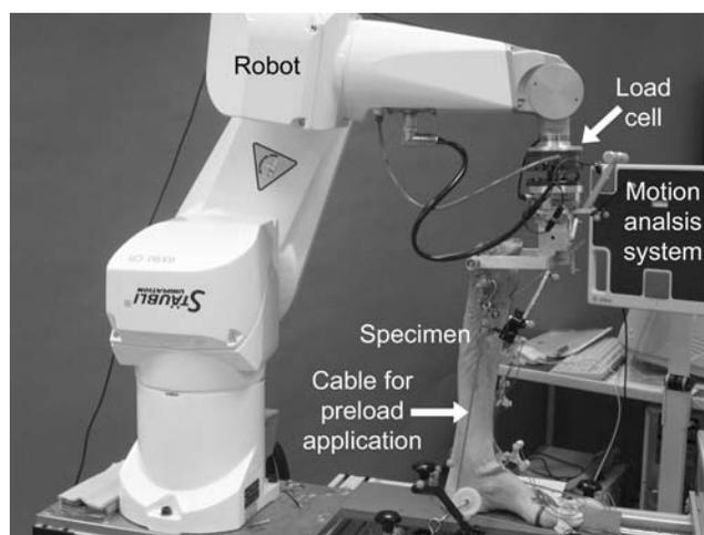
**Fig. 2:** Setting with robot, specimen, and motion analysis system. Specimen mounted is to the robot and footplate. Triaxial transducers of the motion analysis system were fixed to the footplate (black color and in the front) and to the specimen (transparent and at the back of the image or rather the lateral side of the specimen).
