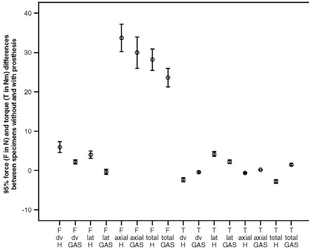
**Fig. 3:** Error bars with 95% confidence interval of force differences between the measurements with a prosthesis (100 cycles) and the measurements of the last (100<sup>th</sup>) cycle without a prosthesis. (F, force; T, torque; H, Hintegra; GAS, German Ankle System; dv, dorsoventral; lat, lateral; total, total resulting).
