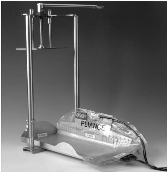
**Fig. 1:** Kraftsimulator Intra-operative Pedographie<sup>®</sup> (KIOP<sup>®</sup>). The custom made mat for force registration is covered intraoperatively with a sterile plastic bag and is placed on the KIOP<sup>®</sup>. The size of the mat is 16 × 32 cm, and it contains 32 × 32 sensors with a sensor size of 0.5 × 1 cm.
